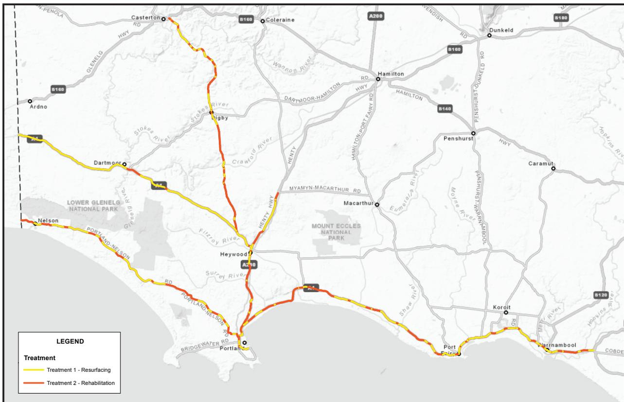
Figure 10: Resurfacing and rehabilitation treatments required under predicted conditions (by 2034), VicRoads
