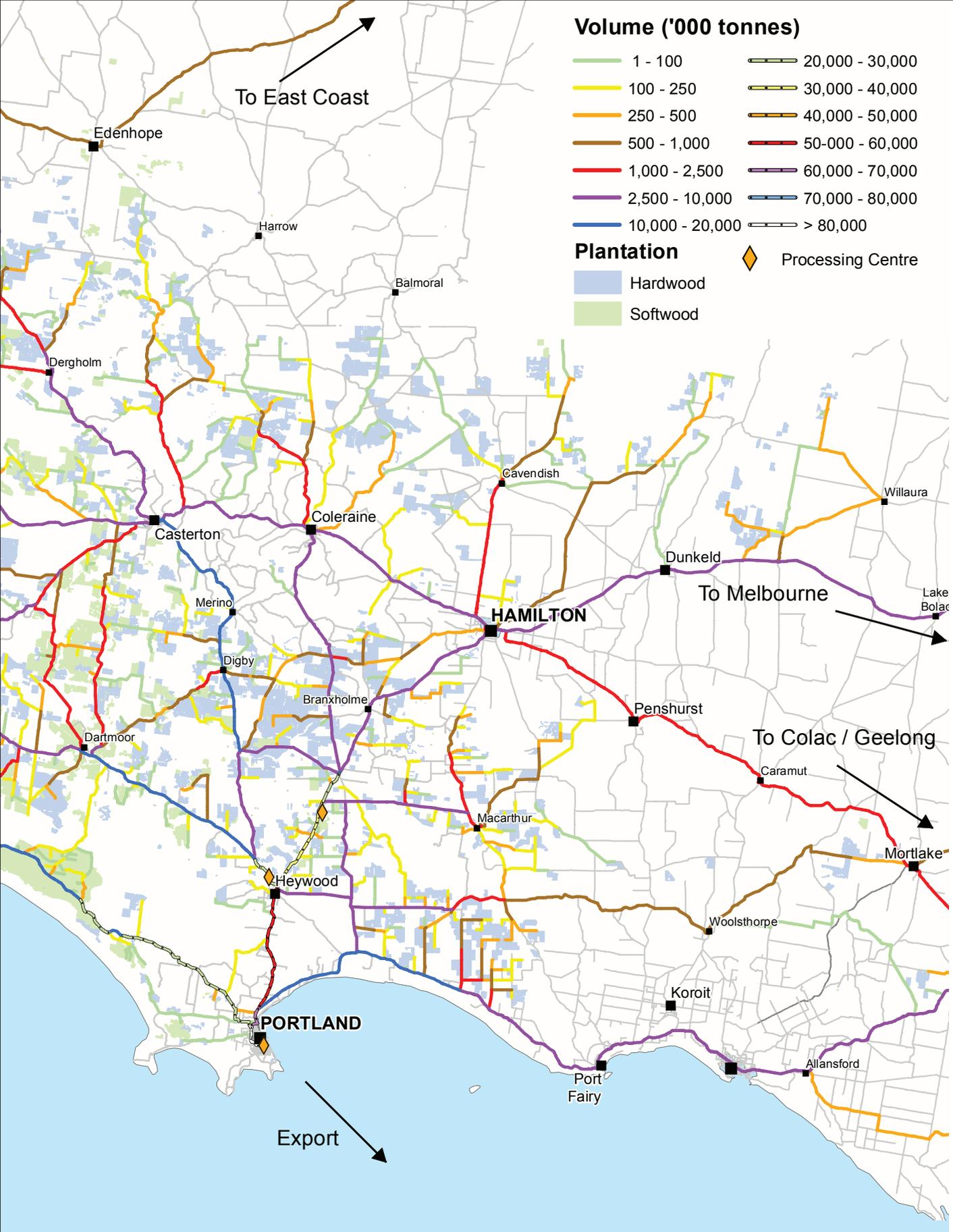
Figure 4: Green Triangle Wood Flow Projections 2015 – 2024, Flying Ant GIS
